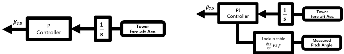
Fig. 4 Tower damper algorithm (left : previous, right : proposed)
