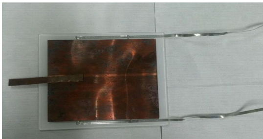
Fig. 1 Fabricated module and copper electrode
