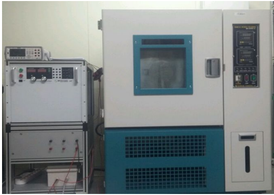
Fig. 3 DC Power Supply and Temperature&Humidity Chamber
