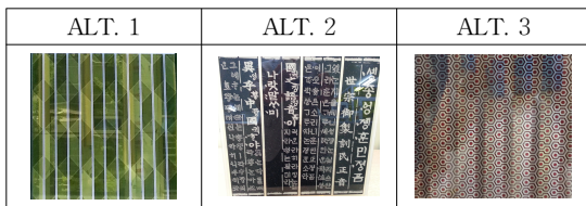
Fig. 8 A plurality of surface structures and pattern of DSC
